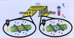
Varying the ionic functionalities of conjugated polyelectrolytes leads to both p- and n-type carbon nanotube composites for flexible thermoelectrics
