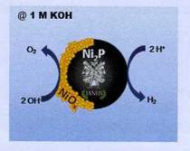
Ni<sub>2</sub>P as a Janus catalyst for water splitting: the oxygen evolution activity of Ni<sub>2</sub>P nanoparticles
