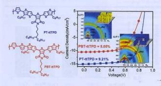
Well-controlled thieno[3,4-c]pyrrole-4,6-(5H)-dione based conjugated polymers for high performance organic photovoltaic cells with the power conversion efficiency exceeding 9%
