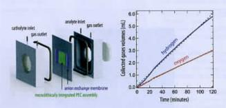
A monolithically integrated, intrinsically safe, 10% efficient, solar-driven water-splitting system based on active, stable earth-abundant electrocatalysts in conjunction with tandem III—V light absorbers protected by amorphous TiO<sub>2</sub> films
