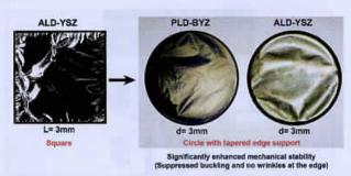
A circular membrane for nano thin film micro solid oxide fuel cells with enhanced mechanical stability
