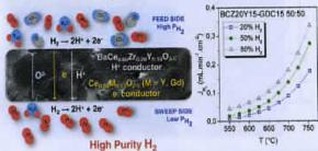
Exceptional hydrogen permeation of all-ceramic composite robust membranes based on BaCe<sub>0.65</sub>Zr<sub>0.20</sub>Y<sub>0.15</sub>O<sub>3 - \(\delta\)</sub> and Y- or Gd-doped ceria
