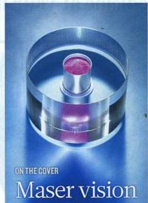
A maser crystal sits inside its sapphire ring. The maser, the microwave-frequency precursor of the laser, could find new applications with the development of a new solid-state maser device. PAGES 285 & 353
