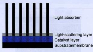
Functional integration of Ni-Mo electrocatalysts with Si microwire array photocathodes to simultaneously achieve high fill factors and light-limited photocurrent densities for solar-driven hydrogen evolution
