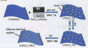
Layer by layer assembly of sandwiched graphene/ SnO<sub>2</sub> nanorod/carbon nanostructures with ultrahigh lithium ion storage properties
