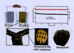
A new configured lithiated silicon—sulfur battery built on 3D graphene with superior electrochemical performances
