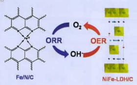
An efficient bifunctional two-component catalyst for oxygen reduction and oxygen evolution in reversible fuel cells, electrolyzers and rechargeable air electrodes
