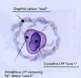
Ultrafast charge—discharge characteristics of a nanosized core—shell structured LiFePO<sub>4</sub> material for hybrid supercapacitor applications
