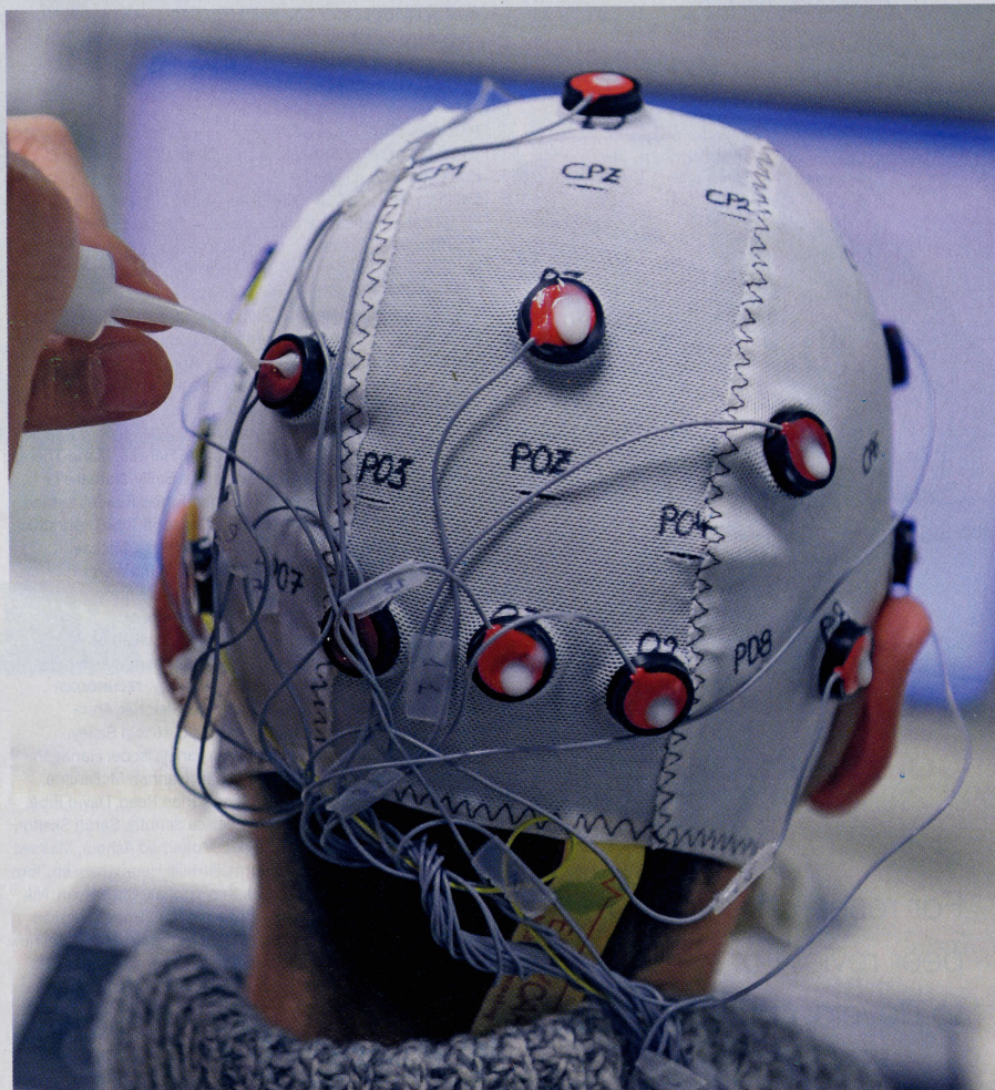
A brain-computer interface that enables the wearer to select symbols on a screen.
